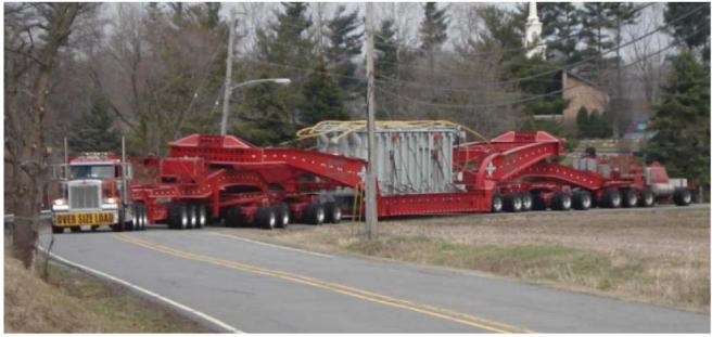
A truck hired to transport a new NIPSCO transformer from Valparaiso to Schererville negotiates a corner. The rig has a driver steering in the front and rear.
