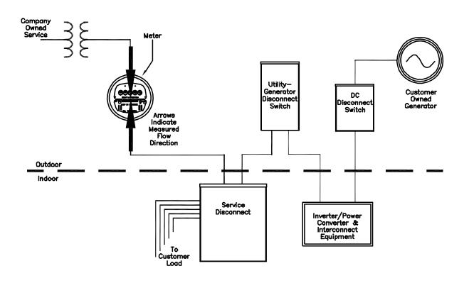
Figure 1 - Typical Residential Solar Installation
