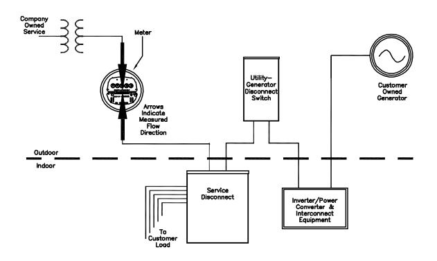
Figure 2 - Typical Residential Wind Installation
