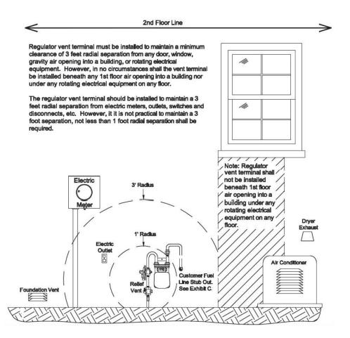
For NIPSCO Electric area only. If you have a provider other than NIPSCO; check with your provider for Electric meter install details.
