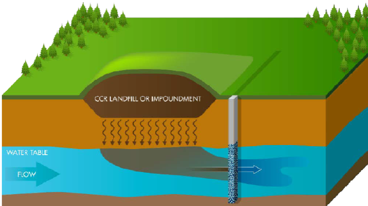
Figure 2-7 PRB illustration showing downgradient PRB, keyed into lower confining unit, and change in concentration as plume passes through PRB media
